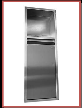
ST-0476 Recessed Waste Receptacle #304 Stainless Steel Satin Finish. With Key. Dimension : 710 x 355 x 105mm. Open Wall : 665 x 305 x 100mm.
