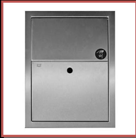
ST-0472 Recessed Waste Receptacle With Flap Door #304 Stainless Steel Satin Finish. With Key. Dimension : 435 x 322 x 105mm. Open Wall : 392 x 280 x 100mm.
