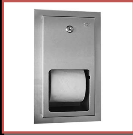
STE-800 SA Recessed Mounted W.C. Roll Dispenser #304 Stainless Steel Satin Finish, With Key. Dimension : 315 x 185 x 120mm. Wall Open : 275 x 145 x 105mm.
