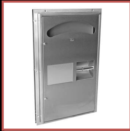
ST-0482 SAD Partition Mounted W.C. Unit (Seat Cover + W.C. Roll + Waste Receptacle With Flap Door, Dual System) #304 Stainless Steel Satin Finish, With Key. Dimension : 810 x 480 x 145mm. Open Partition : 760 x 430mm.
