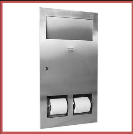
ST-0483 Recessed W.C. Unit (Toilet Paper Holder + Waste Receptacle With Flap Door) #304 Stainless Steel Satin Finish, With Key. Dimension : 745 x 395 x 115mm. Open Wall : 708 x 358 x 105mm.
